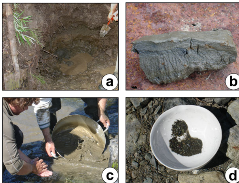
Fig. 3. Field photos: a) the blue variety of clay in place, visible just above the water level; b) a piece of freshly extracted blue clay (length of sample approximately 13 cm); c) the panning operation; and d) residue after panning approximately 20 kg, in an evaporation dish (diameter approximately 10 cm).
